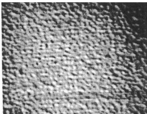
FIGURE 8 TEM micrograph at 20,000X of double SiO deposition.
